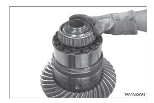
(9) Fix axial roller cage (see arrow) to the sliding sleeve by means of grease.
