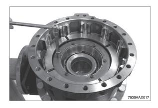
Mount breather valve and press piston out of the brake housing by means of compressed air.
