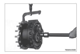
⑥ Fix output to assembly truck.
