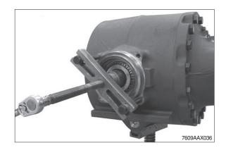
Remove spacer ring and pull the tapered roller bearing from the input pinion.
