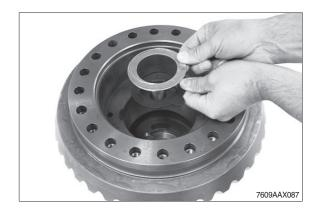
③ Insert axle bevel gear.
