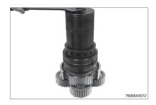
Disengage retaining ring.
