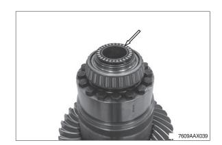
② Pull both tapered roller bearings from the differential.
