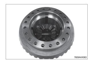
⑤ Remove the second axle bevel gear.
