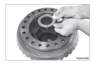
③ Insert axle bevel gear.
